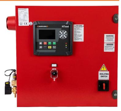
The display and push buttons are used to modify parameters such as the minimum run timer, delay start timer, stop timer, start & stop pressure etc. The display can also optionally show oil pressure, high water temperature, fuel level and water flow (plus others) using a variety of input sensors. There are also several spare inputs and volt free contacts that can be assigned functions.
