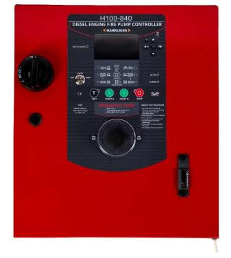
The display and push buttons are used to modify parameters such as the number of flywheel teeth, delay start timer, stop timer, AC failure alarm timer etc. The display can also optionally show oil pressure, cooling water temperature, fuel level and water flow using a variety of input sensors. The controller is also capable of using a pressure transducer instead of a pressure switch for the pump start signal.
