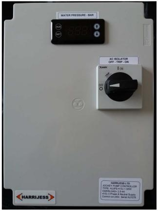
accurately set the start and stop pressures. The set points are password protected. The LED module also allows other useful parameters to be set, such as: Delay start timer, minimum run timer, successive starts timer. The module can also be set with a minimum and maximum water pressure alarm sounder.
